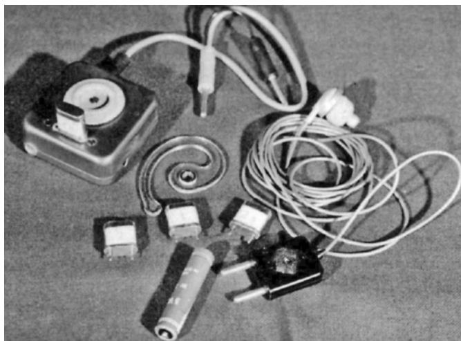
Components of BND SW Converter: converter with crystal inserted; earpiece; three crystals; 3V battery.
