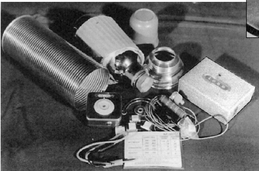
A BND SW Converter with accessories concealed in the bottom of a thermos flask.
